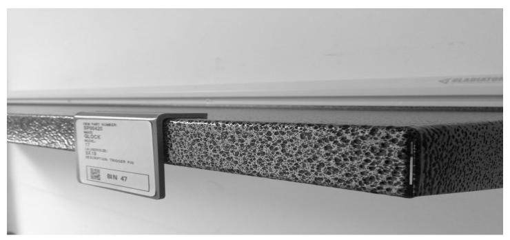
The ArmorerLink® Shelf Label Holder (SLH) is utilized in situations where there is insufficient surface area to affix a label measuring W 2.40 in. x H 2.00 in. (6.09 cm x 5.08 cm). The SLH has double-sided tape on the top and bottom surface of the base for multiple mounting options. The SLH is reusable by replacing the double-sided tape. For permanent installations, the SLH can be mounted using mechanical fasteners.
